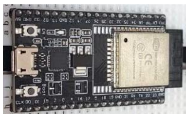
Fig. 3 Photograph of Arudino microcomputer board (Espressif Systems' ESP32 - Dev Kit C).
