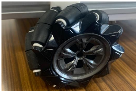
(a) Photograph of used Mecanum Wheel.
