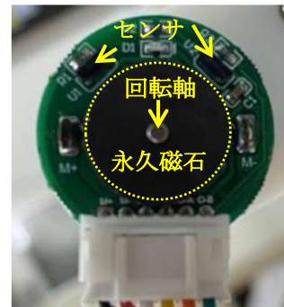
(a) Photograph of magnetic rotary encoder.
