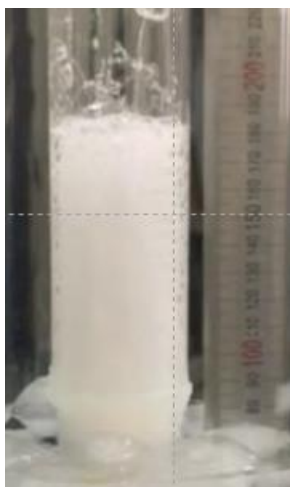
Fig.5 Time variation in foaming height. (65Φ, 2.0L/min (0.01m/s).
