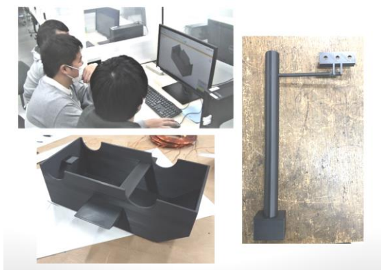
Fig. 5 Photographs of the car body designed with Fusion 360 (upper left side), modeled with a 3D printer (lower left side) and the LED signal (right side).
