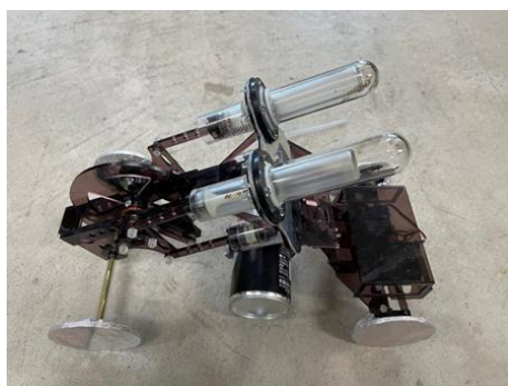
Fig. 1 Structure appearance of Stirling engine car 「Combustion Unit Three version II」.
